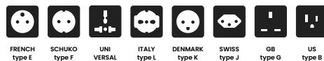
FRENCH type E SCHUKO type F UNI-VERSAL ITALY type L DENMARK type K SWISS type J GB type G US type B
